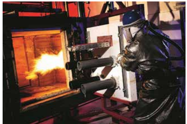
1m 3 furnace tests for some sealants closing penetration gaps. Source: Hilti
