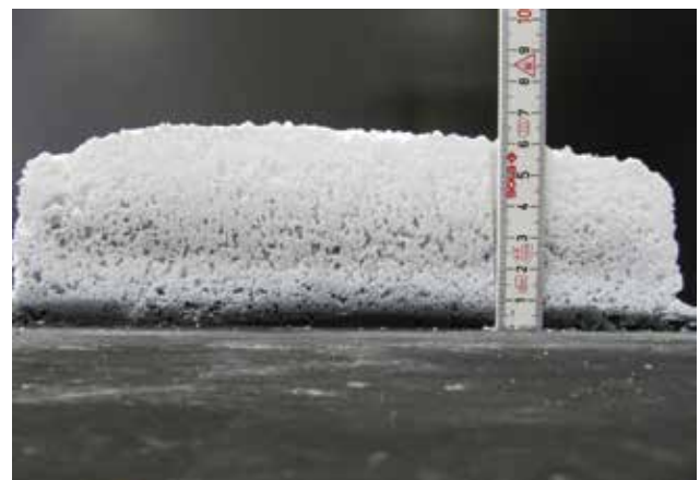
Steel plate coated with intumescent after a furnace test. The coating expands up to 100 times of the dry film thickness.
